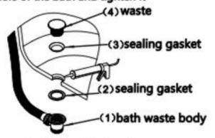
Silicone can also be used during the installation. Once using silicone please leave for 24 hours to dry before use.
