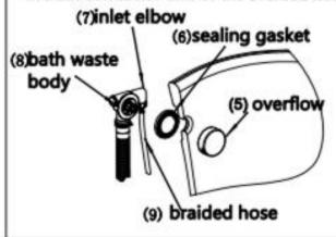
4. fill the bathtub with water and check for leaks. Place the bathtub in the prepared position, connect A side to the drainage pipe. Installation complete
